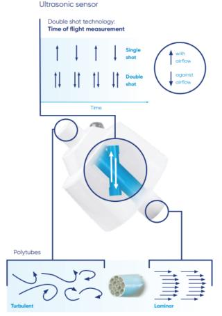
Double Shot Technology measures twice the number of signals across the flow path providing enhanced data resolution and precision.
